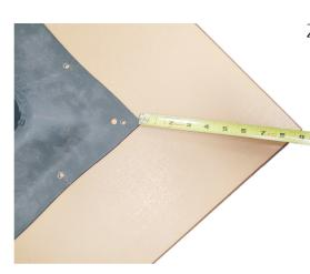
2. Measure from each corner of the spider to the corner of the table. Adjust the base until all 4 corners are equal.
